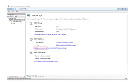
Activate the item "Production machine" (1) and select a path and a file of your choice where PHP should save its log (2). Confirm with "Apply" (3):
